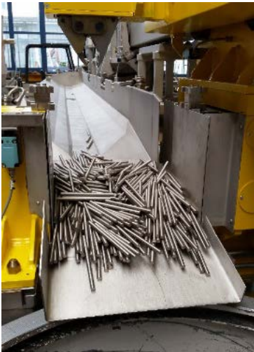
Fig. 5: Short rods at the end of the vibrating process
