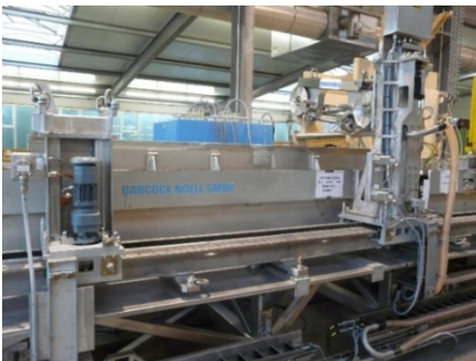
Fig. 9: Saw and feeding unit of the sheath dismantling line
