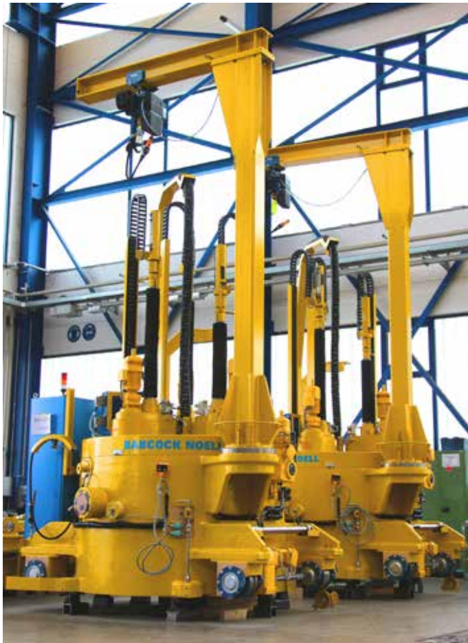
Olkiluoto 3: Filter Changing Machine
