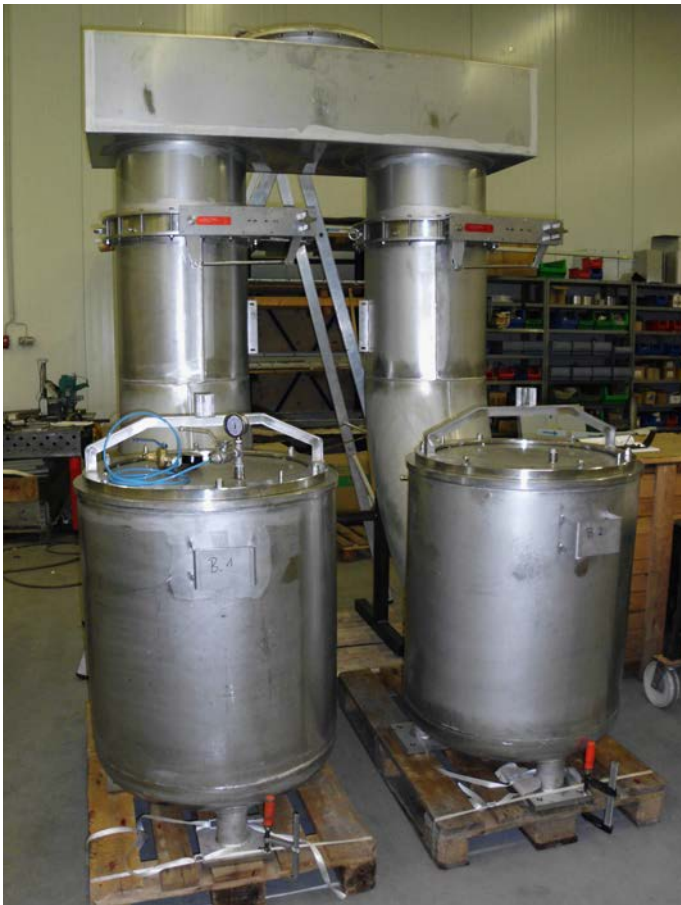
HEPA Filter System for Hot Cells
